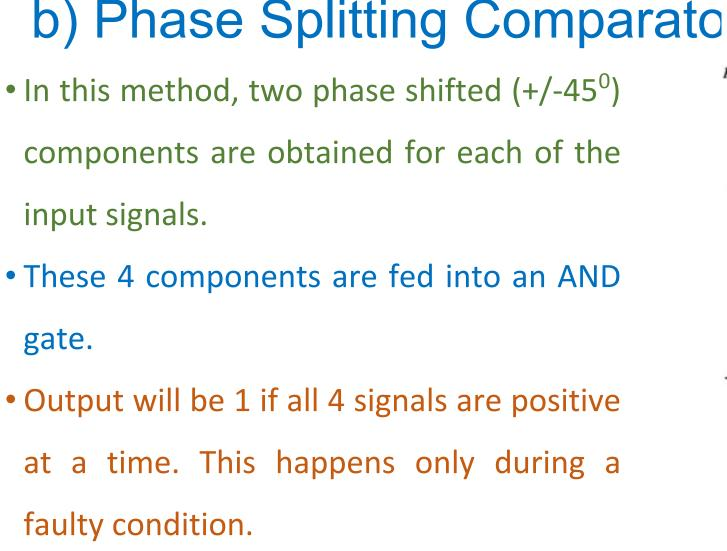
• Output of AND gate is used to trip the C.B
